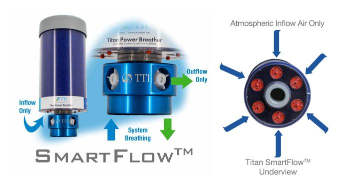
\* Titan SmartFlow PowerBreathers (Titan-XXXX-SF) consist of all check valves positioned inward to exclusively inhale from the atmosphere, therefore must be used with the Titan-SF-A1 (1" FNPT) or Titan-SF-A2 (2" FNPT) SmartFlow Adapters to exhale all air out of the system.
