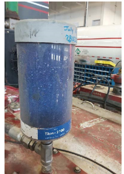
TTI Titan 2100, Serva Twin Pump, Passenger's Side—Shown at 613 Service Hours
