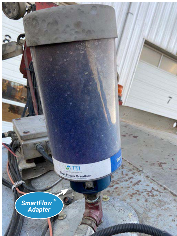
TTI Titan 2100 with SmartFlow™ Adapter, Frac Unit #1—Performing Well After 400 Service Hours.
