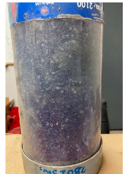
TTI Titan 2100, Serva Twin Pump, Passenger's Side—End of Test After 1602 Service Hours
